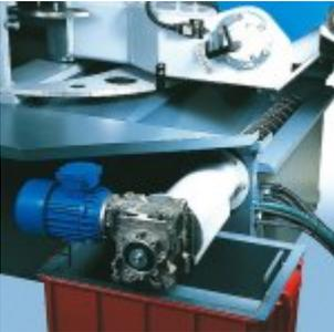
**Screw chips conveyor - Standard equipment**
